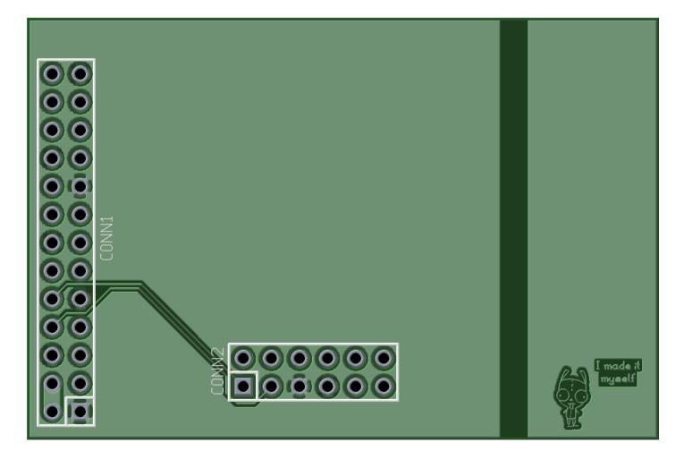
In this example PCB I have connected the GPIO SPI TX/RX pins that would then be connected to a PIC or Atmel chip. In order to use these pins and have access to the port you only need to disable the Linux serial console that by default uses these pins as ttyAMA0.
